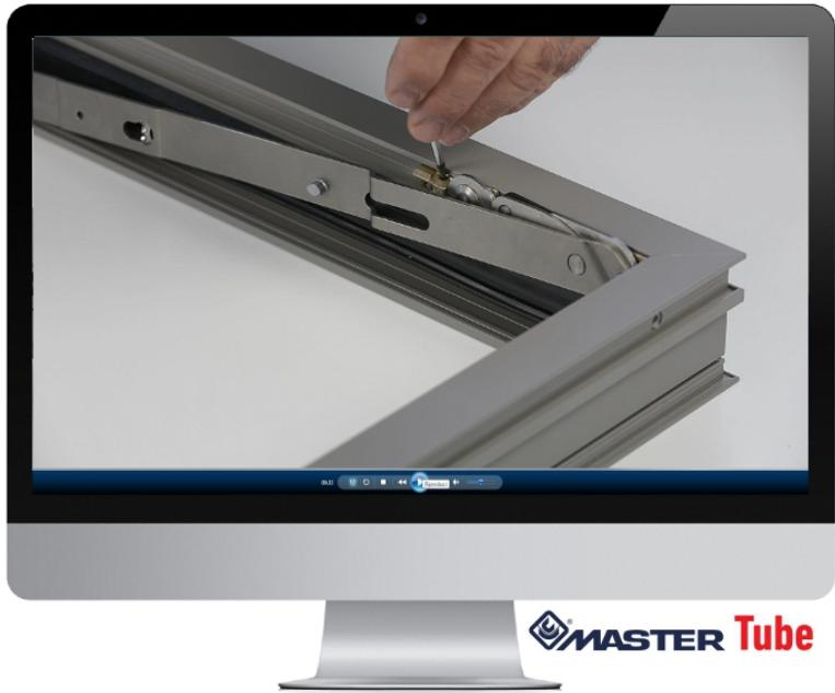
**WEEN HIDE 180 Video tutorial is online on MasterTube: the Master solution for tilt & turn system with 180° opening angle**
